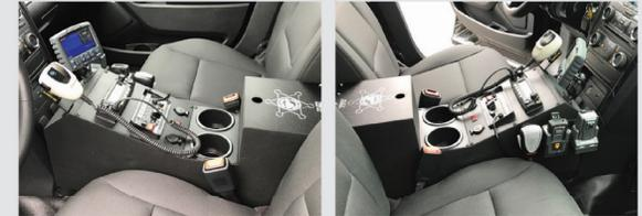
Custom built equipment consoles to fit any customer requirement. Welded steel construction and powder coated finish for maximum durability. The entire process from design to finished product is done in house at our Morgantown location.
