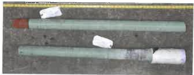
Failed High Tensile (150ksi) Steel Anchor Bar
