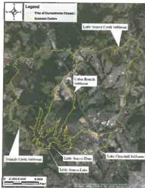
Watershed Model Example for an Earth Embankment Dam similar to Pierce Lake Dam.
