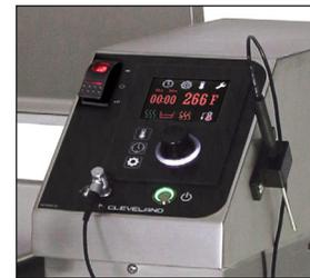
easyDial Control Panel with Core Temperature Probe
