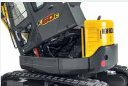
Forward tilting cab on E60C eases maintenance access
