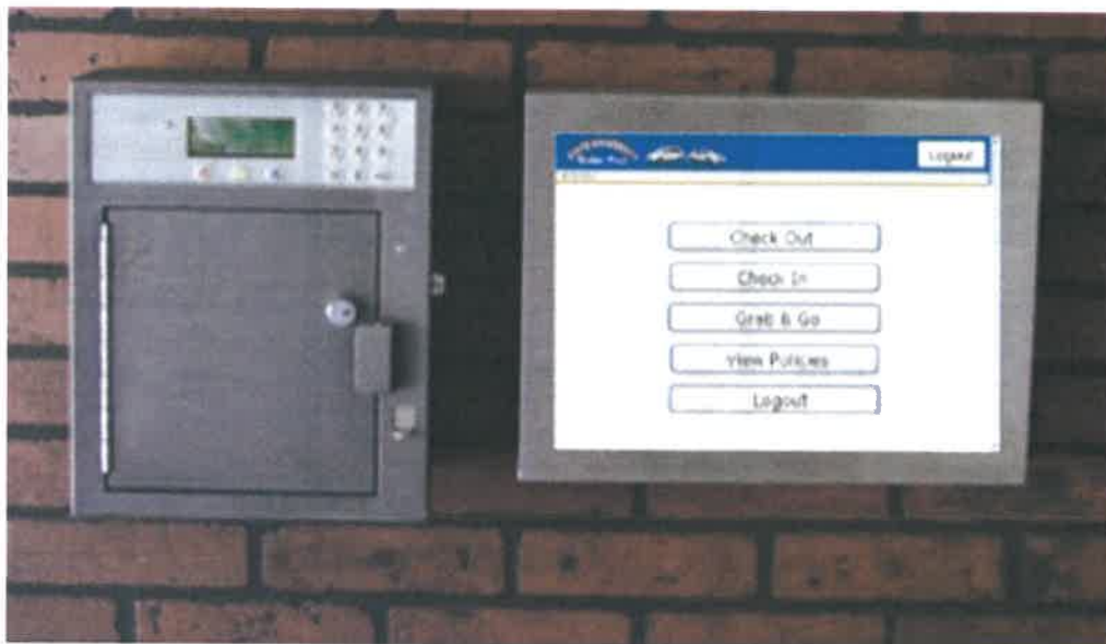
A standard self-service motor pool consists of a key control device (on left) and a full-color, touch-screen kiosk (on right)
