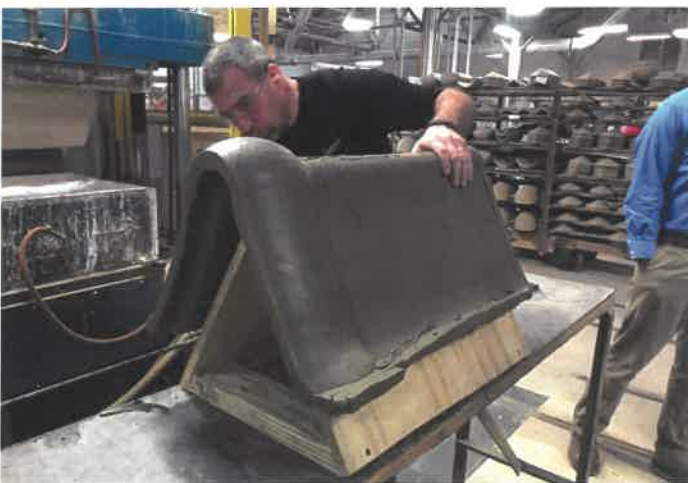
PWWG coordinated a tour with the County's project team of the Ludowici clay tile factory to observe the manufacturing process for specialty tiles used for the Courthouse re-roofing.
