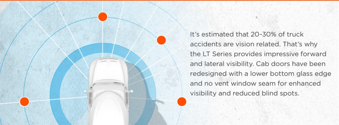
It's estimated that 20-30% of truck accidents are vision related. That's why the LT Series provides impressive forward and lateral visibility. Cab doors have been redesigned with a lower bottom glass edge and no vent window seam for enhanced visibility and reduced blind spots.
