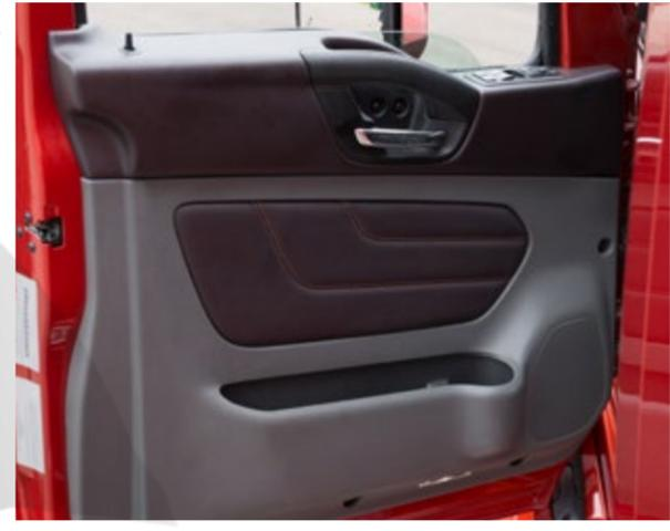
All-new door panels help increase hip and elbow room while providing a more comfortable place to rest your arm. The new full-grip interior handle makes doors easier to open and close, while new door pockets offer easier access to the driver's log or manifest.
