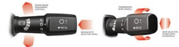
▶ The innovative new shifter is mounted on the steering column, allowing you to easily reach and smoothly operate shifting and engine braking while keeping your eyes on the road and your hands on the wheel.
