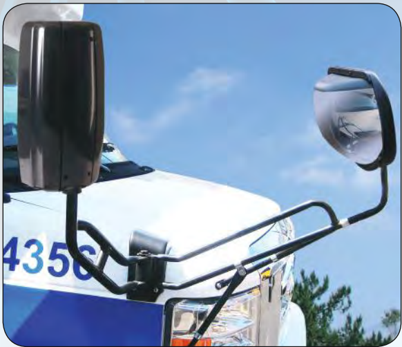
AccuStyle® Rearview & Eye-Max® LP Crossview Combination Assembly
