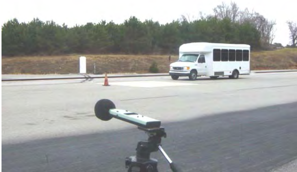
TEST BUS UNDERGOING EXTERIOR NOISE TESTING
