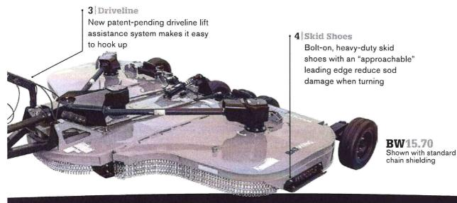
\*NOTE: Woods Batwing\* models pass all applicable safety standards for thrown object and blade contact without chain shielding. However, if these units will be used in areas where the possibility of thrown objects could be hazardous to persons or property, it is strongly recommended that optional chain shielding be used for extra protection.
