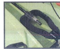
Single levelling rod with floating hitch
