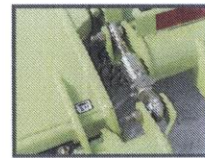
Greaseable adjustable turnbuckles for parallel levelling
