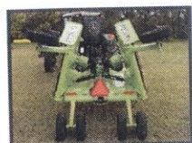
Narrow transport over-centering wing design
