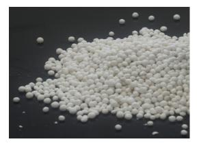
Cryotech CMA is a minimum of 96%, by weight, hydrated calcium magnesium and other acetates with less than 4%, by weight, water-insoluble material. Notice the uniform appearance of the pellets. This is Unipel technology, a unique process which ensures each pellet receives the same distribution of active ingredient. CMA provides the most protection from concrete spalling and is less corrosive than tap water.
