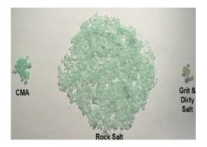
This product that contains calcium magnesium acetate blended to less than 20%, by weight. An analysis, performed by an independent laboratory shows this blend to be less than 5% CMA, by weight, providing little or no protection against concrete spalling and corrosion.
