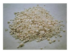
Cryotech CMA40 is Cryotech CMA at a concentration of 40% by weight blended with a high quality grade of salt. Notice the amount of Cryotech CMA pellets in this blend. The more CMA in the blend the better the protection.
