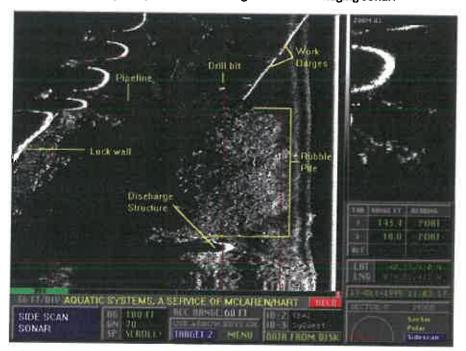
Side scan sonar image illustrating location of drill bit in relation to subsurface pipeline, discharge structure and rubble pile, positioned upriver from Lock & Dam 2 on the Monongahela River.
