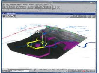
Kimball hydrogeologists prepared a simple 3D model, depicting the mine workings, the overlying strata, and locations of overlying coal seams with respect to the valley of Fourmile and Monastery Runs. Based on an analysis of the model, a report was developed identifying alternative methods for collection of the artesian flows for treatment in the MRIP. The report discussed each alternative and included a list of recommendations, including reuse of the current location.
