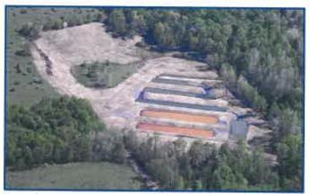
Kimball prepared a site remediation plan for the Laurel Run #2 abandoned mine land site in Indiana County, PA. The project included aerial photography and mapping of the site limits, geotechnical investigations of the existing spoil material, installation of several borehole/monitoring wells above the highwall, design of the acid mine drainage (AMD) remediation technique, and preparation of a construction bid package, as well as periodic site observation during and after construction.
