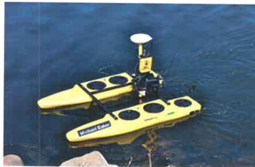
Michael Baker owns a HyDrone bathymetric system and has used it on numerous mine ponds.
