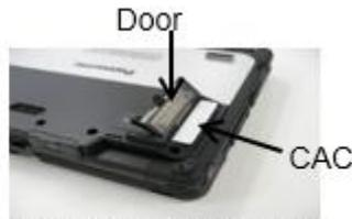
The entire card is placed in the inside of the cover to improve water resistance.
