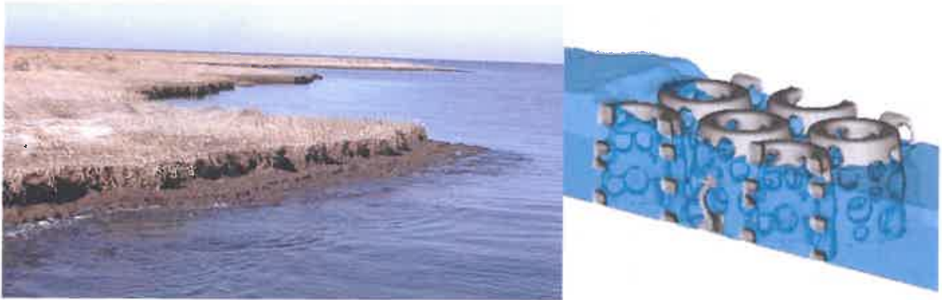
Bio-engineered oyster reef demonstration project in southwest Louisiana (left) used modeling tools (right) to optimize design.
