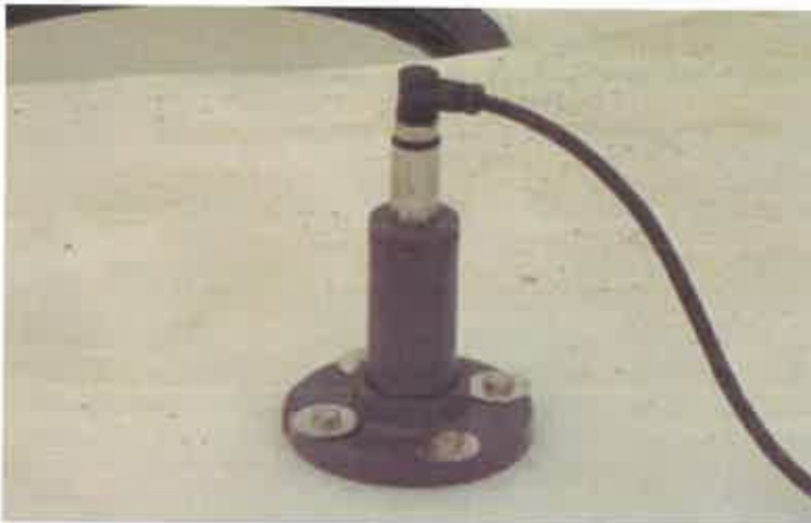
PT assembly – pipe, pipe cap, mounting flange, PT and PT connector shown
