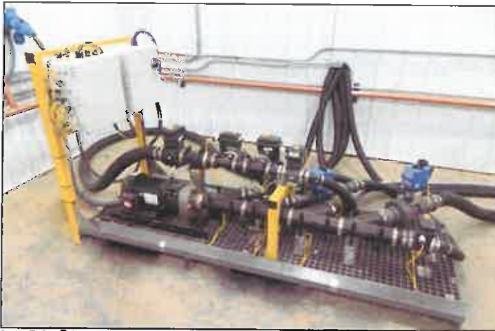
AccuBrine ® blend truck loading & blending skid
