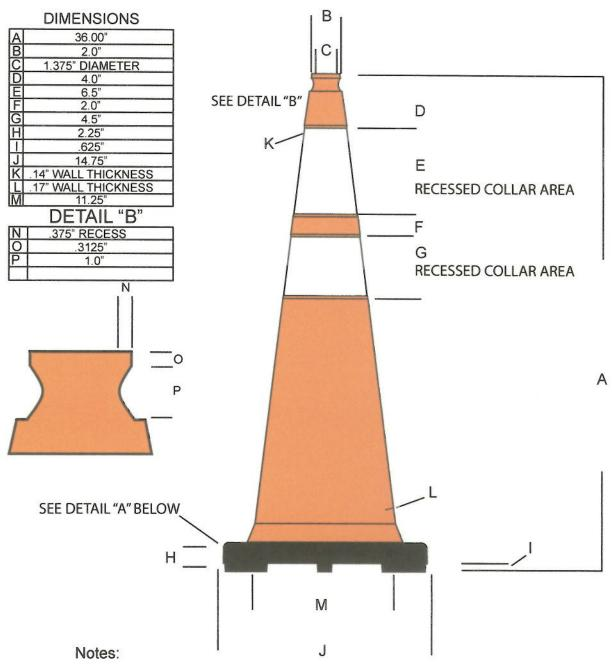
Conical section manufactured from 100% recyclable flourescent orange PVC Base manufactured form 100% post industrial recycled black PVC
