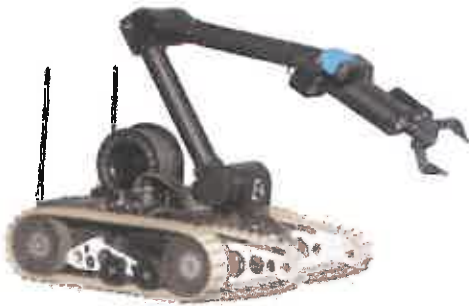
CAMELEON - modular mobile EOD robot
