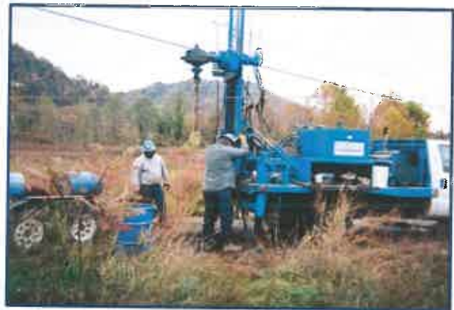
Environmental Sampling for an Underground Storage Tank Site Investigation
