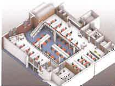
Test fit with the Revit 3D model to estimate capacity and operations with adding a Mezzanine.
