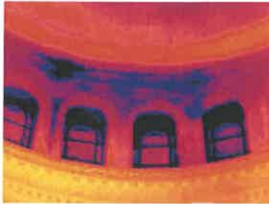
Investigation Phase at Church Interior, (left) Thermal imaging detects trapped moisture (right)
