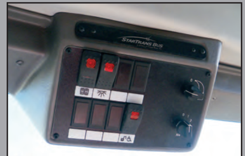
Driver's switch panel conveniently located within view of the road and not on the engine cover
