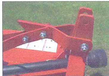
Floating Hitch for uneven terrain
