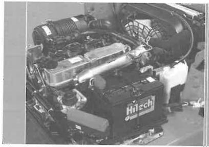
Engine Protection: Regulated by the Vehicle Control Module, the Engine Protection System keeps the truck running at destrable levels while helping to prevent damage to the torklift, saving you money if any of the vital fluids become critically low, RPM levels are automatically lowered and the operator is immediately notified by a light on the dash display.
