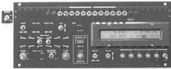
Control panel with computerized application rate control and spray controlled in 1' increments.
