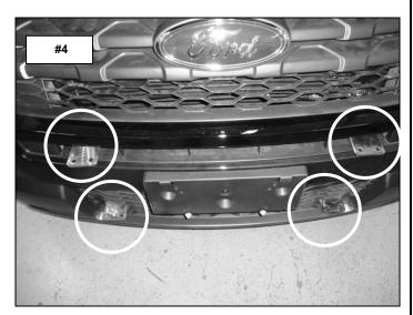
**Step-7** Attach each of the passenger side extension brackets to the main bracket using (2) 3/8" x 1" hex bolts, (2) 3/8" lock washers and (2) 3/8" hex nuts, (Photo 5). Leave the nuts and bolts loose for final adjustment. Repeat this step for the driver side, (Photo 6).
