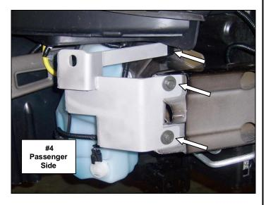
**Step-4** Refer to the installation instructions included with the push bumper (#5039) to notch the bumper insulator and complete the push bumper bracket installation. **Picture #5**
