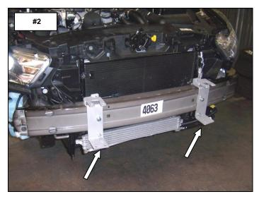
**Step-2** Beginning with the passenger side, remove the (2) 13mm head bolts securing the end of the steel impact beam to the frame. **Picture #3**
