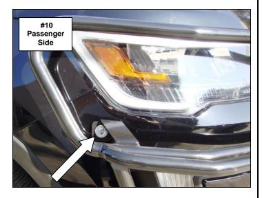
Step-11 Align the push bumper and brush guard assembly with the vehicle and tighten all nuts and bolts.
