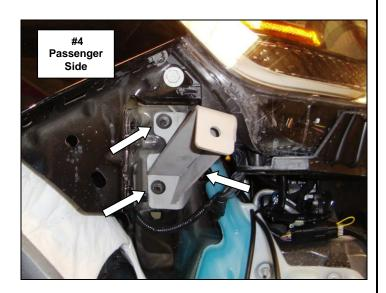
**Step-4** Reposition the front bumper fascia on the vehicle and install the hex bolts and plastic connectors securing the top of the fascia, install the hex bolts securing the fascia to the front fenders and the hex bolts securing the bottom of the fascia. Tighten all bolts. **Note:** Do not install the screws securing the fender liner and fender molding to the front bumper fascia.
