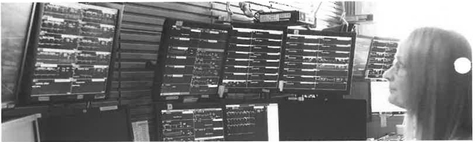
Remote displays in cockpit with KVM, audio, and mounts.
