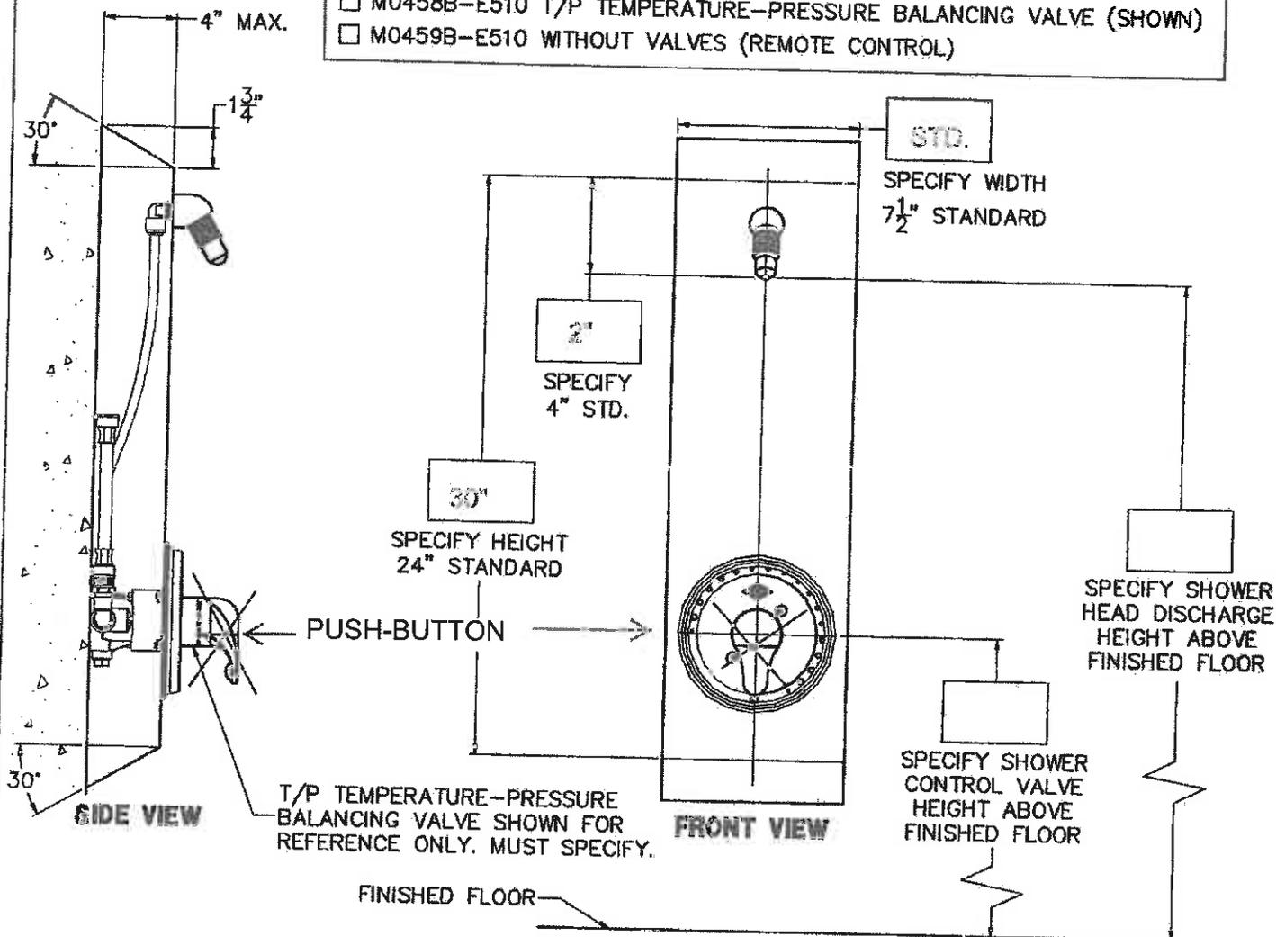
**ACORN M0450-E510 APEX SURFACE-MOUNTED SHOWER MODIFIED WITH SPECIAL HOUSING**
