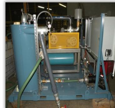
*SVE skid with vacuum pump, condensate tank, and panelboxes*
