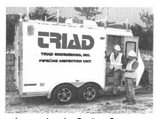
the necessary equipment to perform a thorough and comprehensive Sanitary Sewer Evaluation Study including Closed Circuit Television Camera Systems (remote control and cable driven), flow meters and smoke testing equipment.
