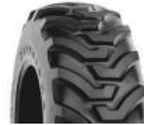
R4 - Industrial-tread Excellent utility tread; gives long life on hard surfaces like pavement and provides a smoother ride while roading.
