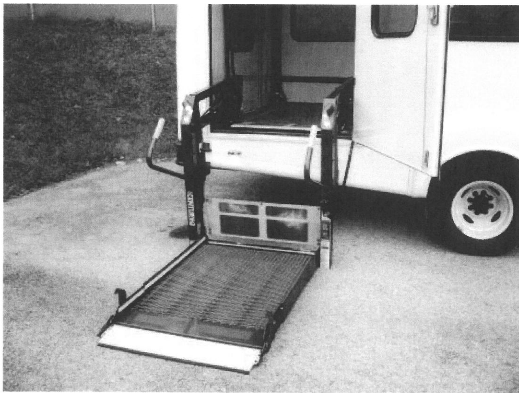
GOSHEN COACH MODEL 2013 IMPULSE EQUIPPED WITH A BRAUN MODEL NCL919FIB-2 HANDICAP LIFT
