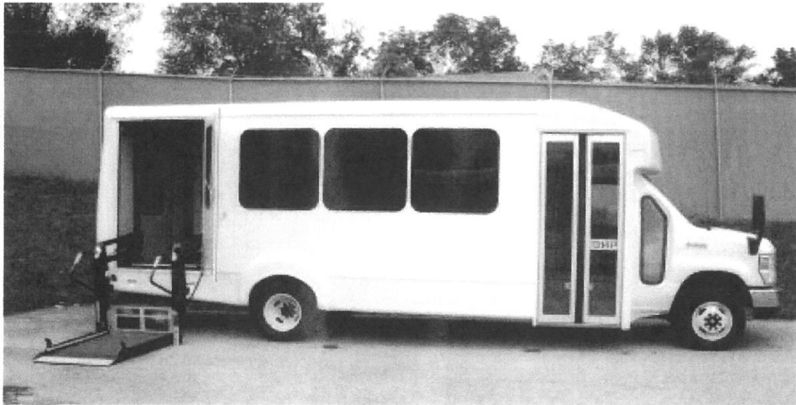
GOSHEN COACH MODEL 2013 IMPULSE EQUIPPED WITH A BRAUN MODEL NCL919FIB-2 HANDICAP LIFT
