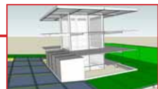
Museum of Contemporary Art — Los Angeles, California Aluminum and Glass "CUBE" display case. Extensive seismic analysis and anchor design. Mass-sensitive, optimized model.
