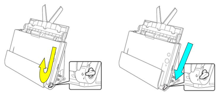
U-turn feeding: Set the lever at the upper position ><Straight feeding: Set the lever at the lower position>
