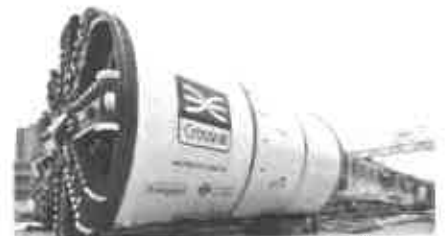
Crossrail's six tunnel boring machines weigh 1,000 tons each and are being used to expand London's subway system.
