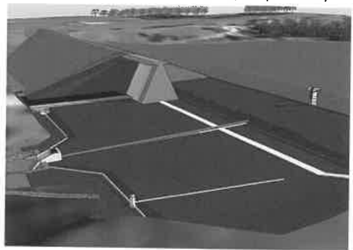
Lost River Site No. 16 Riser Rendering. Gannett Fleming designed the structure to retard the runoff from a 10-day duration, 100-year frequency storm without discharge occurring in the auxiliary spillway.
