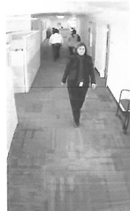
Vertical Field of View with Corridor Mode
