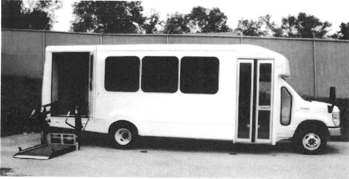
GOSHEN COACH MODEL 2013 IMPULSE EQUIPPED WITH A BRAUN MODEL NCL919FIB-2 HANDICAP LIFT
