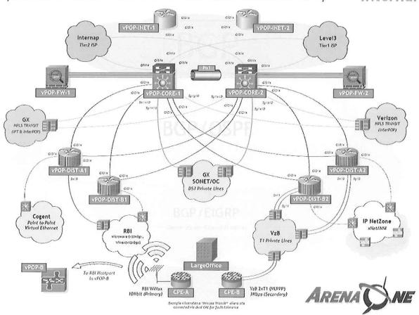
Arena One maintains a fully redundant network core, VoIP application servers, and session boarder controllers. There are no single points of failure in the network, facilities, application, or voice delivery infrastructure.
