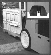
Exclusive precision load positioning on incline capability minimizes the likelihood of product damage from unintended load contact. Dual steer tires, with hydraulic actuated rack and pinion steer axle, provide precise, reliable control for maximum performance.
