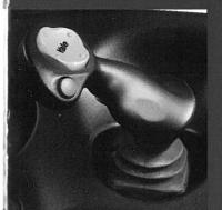
The multi-function control handle has been designed for low effort, single hand control of travel direction, speed control, hydraulic functions, and horn actuation. The built-in palm rest allows the hand to rest comfortably on the handle while providing support to the arm.
