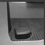
The spacious operator compartment has a fully padded floor with 3/4" thick rubber mat and shock absorbent "isolated" floor design that reduces operator fatigue. A low 7" step height provides easy entry and exit.
