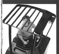
The overhead guard is a three post design to provide excellent visibility for maximum operator productivity.
