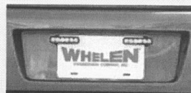
IONBKT1 License plate mount and two IONJ.
