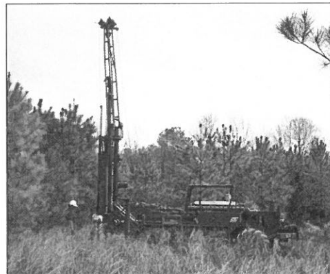
CTL's ATV can drill in rough terrain
