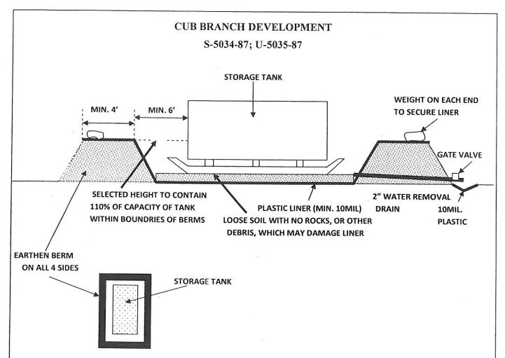
\*A two inch (2") water removal drain shall be located at the lowest point in the bottom of the containment volume. It shall connect to a normally closed gate-valve outside the dike. The gate valve is manually operated and protected from unauthorized operation. Rainwater contained within this dike shall be examined prior to release to ensure that harmful quantities of fuels and lubricants are not discharged.
