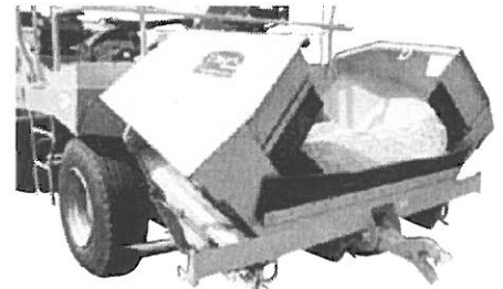
Folding Bat Wing Rear Receiving Hopper provides increased aggregate capacity and easy clean out of hopper. Facilitates easy change of aggregate types.
