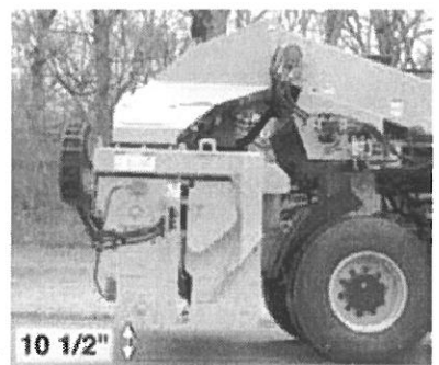
Front hopper raise and lower system to clear obstacles. Easier loading.
