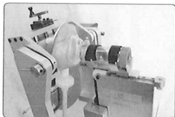
VHC test facility: the facemask on test was loaded onto the face with a fixed 1.6 kg force
