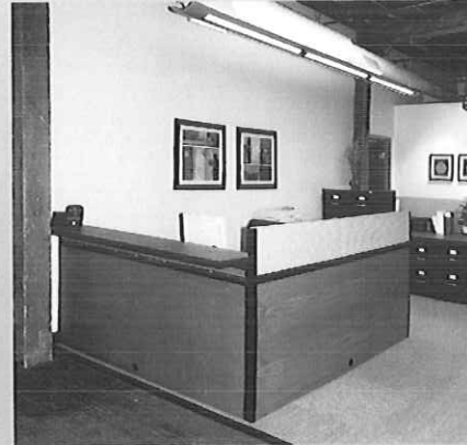
WAREHOUSE TO OFFICE BUILDOUT (Doors Reused as Desks) Charleston, West Virginia
