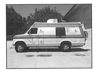
Although most vehicles the size of an SUV or larger can be used for emergency response vehicles, FTI's current vehicle is based on a Ford E350 retrofitted medical van. FTI's ECRV can include a fully integrated high-performance satellite communications link; both wired and wireless telecommunications gear including a digital phone, GPS, laptops, and even video surveillance equipment; and multiple power interfaces for a generator or other standby power.
