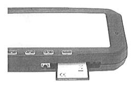
All DVM models use a Compact Flash (CF) card form factor memory module to record the video data. The Compact Flash cards are completely solid state, eliminating most all of the drawbacks to video systems that use hard disk drives to record and store their data (moving parts, cooling, performance degradation over time, etc.)
