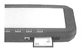
All DVM models use a Compact Flash (CF) card form factor memory module to record the video data. The Compact Flash cards are completely solid state, eliminating most all of the drawbacks to video systems that use hard disk drives to record and store their data (moving parts, cooling, performance degradation over time, etc.)
