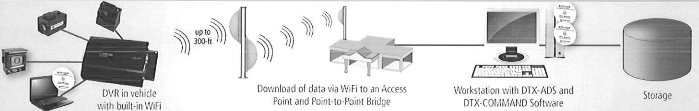
Diagram 3 - Model DTX-SYSTEM-1 with greater than 300-ft wireless WiFi download to back-office
